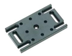
Mini-post bases are thin plates of aluminum which have an M4 threaded hole for the mounting of a mini-post or mini-post holder. They also have slots or clearance holes for mounting onto a mini-baseplate. Three types are offered: a simple base with slotted holes either side, an adjustable base with a single 15mm long slot, and a large base which will accept either a mini-post or a mini-stage. The bases are 5mm thick. See drawings on opposite page.
