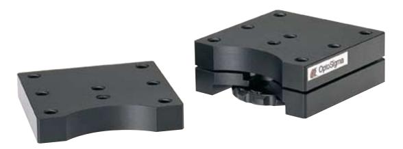
Kinematic bases use three balls which locate against a flat, a cone and a vee groove. This method of mounting ensures precise positional replacement of the base. The lower plate may be attached to a standard breadboard hole pattern and the top plate will accept stages or other mounts. By using a number of separate top-plates it is possible to exchange samples with a high degree of precision. The thumbwheel protruding from the bottom plate is used to secure the top plate in position.
