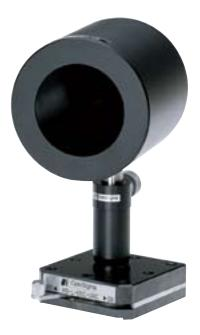
Laser beams passing into the aperture of these beam dumps are quickly dissipated and absorbed within the body of the dump. A ribbed conical design ensures that incident laser energy will not emerge to interfere with wanted parts of the beam or to cause inadvertent damage. Two sizes, 10mm and 52mm cover most laser beam sizes. The bases are threaded 8-32 or M4 for attachment to posts or pedestals.
