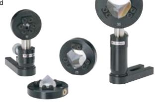
Retro-reflectors are some of the most difficult components to support and align. With the face perpendicular to the optical axis there is no clear reference surface. These holders make it simple to hold and align retro-reflectors. Once mounted in these rings they may be treated like any other component. Individual holders are offered for each of the most common diameters. The base of the holders are threaded 8-32 or M4 for inch or metric post or pedestal base mounting.
