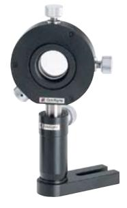
Lenses may be mounted directly into these holders by means of the retaining ring provided. The optical axis is easily adjusted in two axes by means of the fine pitch, 50TPI (0.5mm) adjusting screws which protrude from the side of the holder. These adjusters operate against a springloaded plunger which will retain the lens in position, once set. The holders may be attached to a post or pedestal base by means of an 8-32 or M4 screw.
