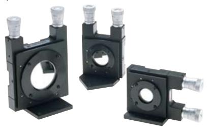
Two precision micrometers are mounted vertically within the width of the mirror mount. They are easily reached from above without having your hand block the beam. The mirror can be adjusted in two axes of tilt. The micrometers facilitate extremely precise adjustment. Anti-backlash springs maintain the mirror in position and provide for repeatable settings.
