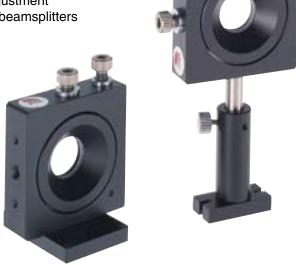
Mini-beamsplitter mounts are cut away from the component more than mirror mounts. They permit a 45 degree incident beam to pass unimpeded through the mount. For this reason they are slightly larger than the mini-mirror mounts. These mounts accommodate only 15mm diameter beamsplitters of thickness up to 2mm. This provides a 6mm diameter clear aperture at 45 degrees. They have two top-projecting screws to provide  $\pm 2$  degree of tilt over two axes.
