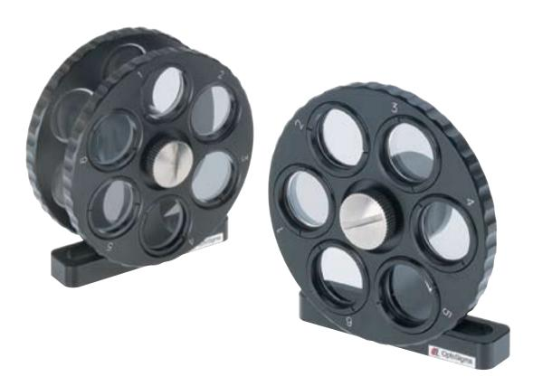
Our new indexed filter wheels contain a set of neutral density filters. These pre-mounted filters are available in complete 2-wheel or starter 1-wheel versions. Each filter wheel holds six, 1 inch (25mm) filters and is mechanically indexed with detents for ease of adjustment.
