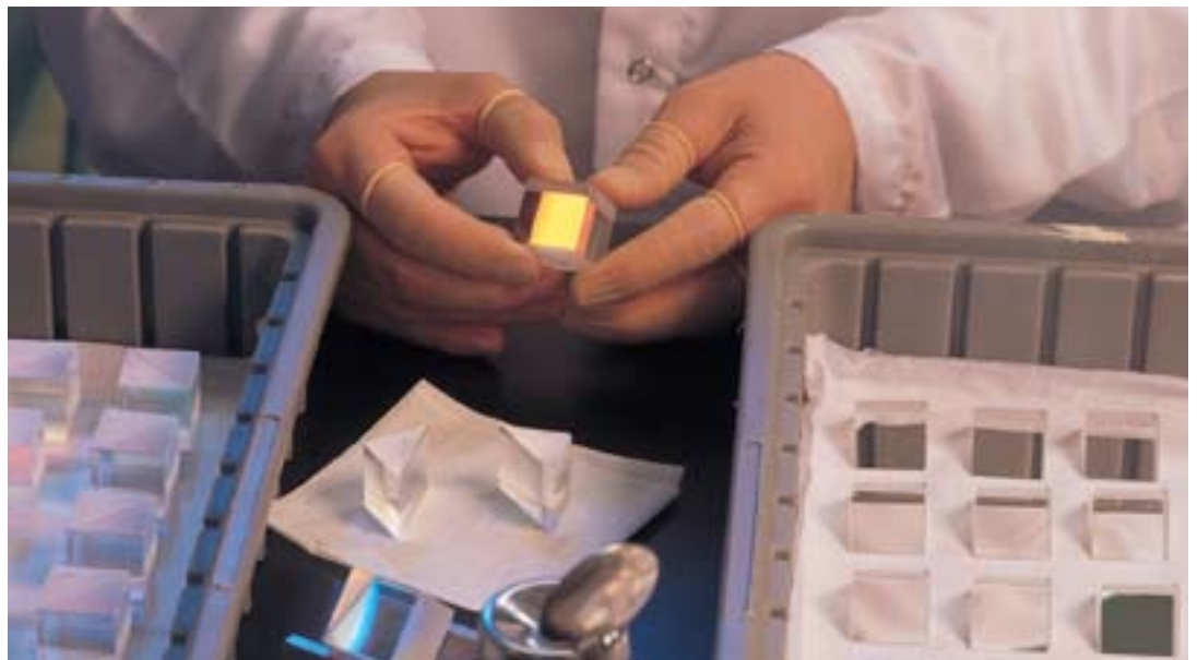
Our cube beamsplitter assembly takes place in a clean room environment to ensure high quality.
