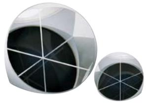
These retro-reflectors are extremely precise providing an exact 180 degree deviation within a 2arcsec tolerances. This enables them to be used for high precision applications or with lasers over very long distances. These "angle insensitive" mirrors have numerous uses in alignment and metrology. Our retro-reflectors come standard with a broadband AR coating on the face. Optional black paint protected silver may be specified for the legs.
