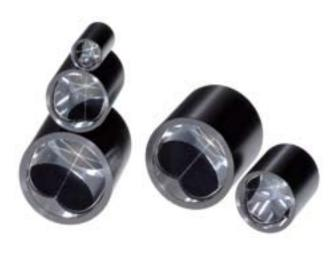
The precision assemble of the flat mirrors in the hollow retro-reflectors insure highly accurate beam deviation. Each retro-reflector is assembled in a black anodized aluminum mount. These "angle insensitive" mirrors have numerous uses in alignment and metrology. Our retro-reflectors come standard with protective aluminum for use in the visible spectral region.
