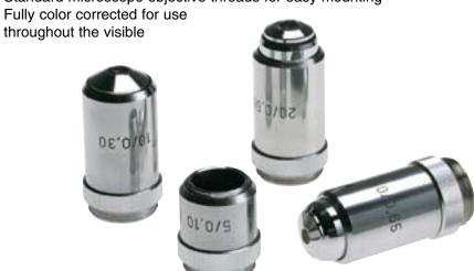
Microscope objectives are ideal for use as focusing lenses for low power lasers such as HeNe, HeCd, and N2. We offer a selection of precision achromatic objectives covering a range of numerical apertures. They are housed in conventional microscope barrels and fitted with a standard RMS microscope thread. The lenses are Anti-Reflection coated.
